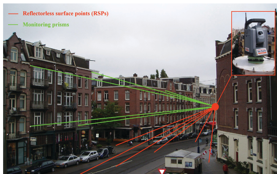
Figure 1. A Reflectorless Robotic Total Station (RRTS) measuring RSPs and prisms.
